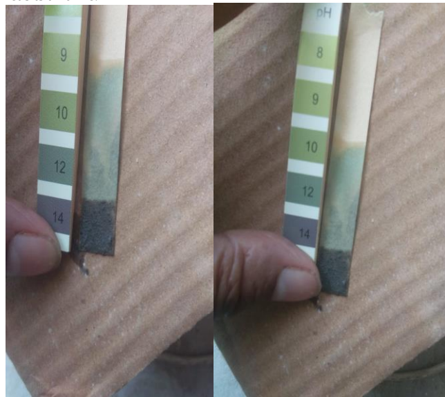
Plate no. 4 A: p H of soil Plate no. 4 B: p H of water , from Dhanauri Wetland during survey.
